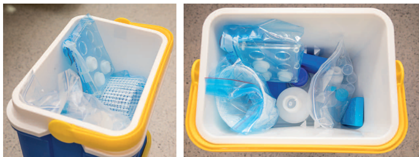
Image 5. Double bag DGT assembly and other needed material in cooler box (Source: ITC).
