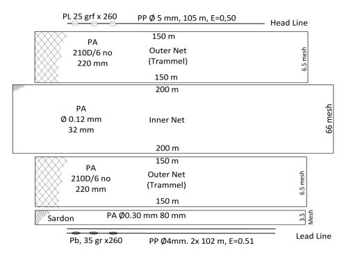
Figure 2. Technical features of the trammel nets used in the study
